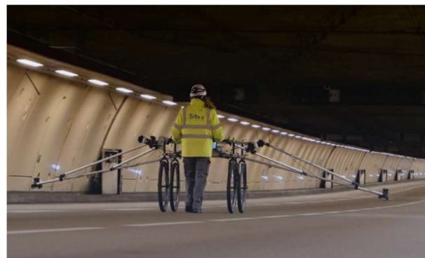
Figure 2 Adaptation of ScanTubes® system to large tunnels
